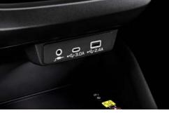
Front USB Ports (Type-A and C\*2) and Rear USB Power Ports\*2
